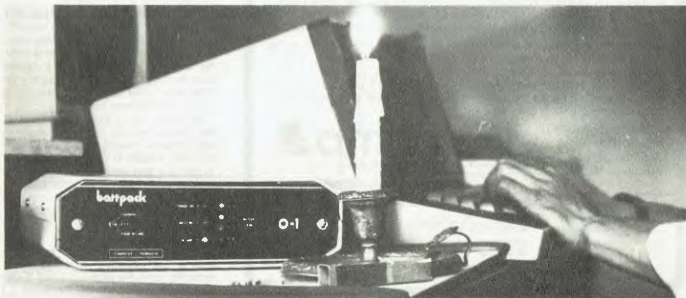
The Osborne's Battpac — for working in the field, or for when the power fails.
